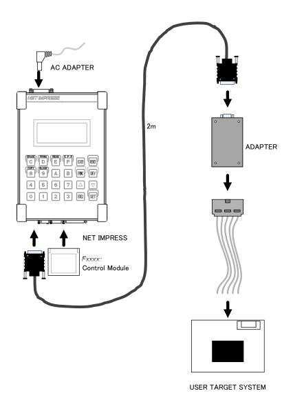
The figure below illustrates the example of connection on a circuit.
